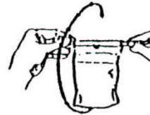
F. Whirl the bag 5 complete revolutions and twist the ends of the wire together 2-3 times.
